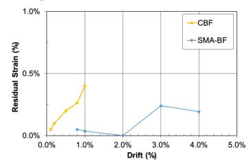
Figure 5:Residual strain in the brace after the last cycle at each drift level
