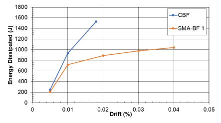
Figure 6: Energy dissipated over a range of drift levels
